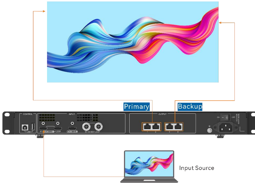
Figure 5-22 Ethernet port backup connection
